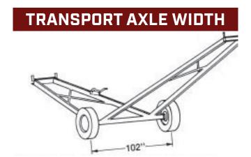
(From center of tire to center of tire - outside width will vary depending on tire width) Safety cable removed for display purposes only.
